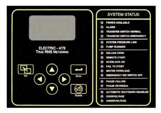
**Description**—Firetrol® FTA1500 Primary Resistance Fire Pump Controllers use resistors in the line to reduce line voltage when starting the pump motor. The controller monitors, displays and records fire pump system infor-
